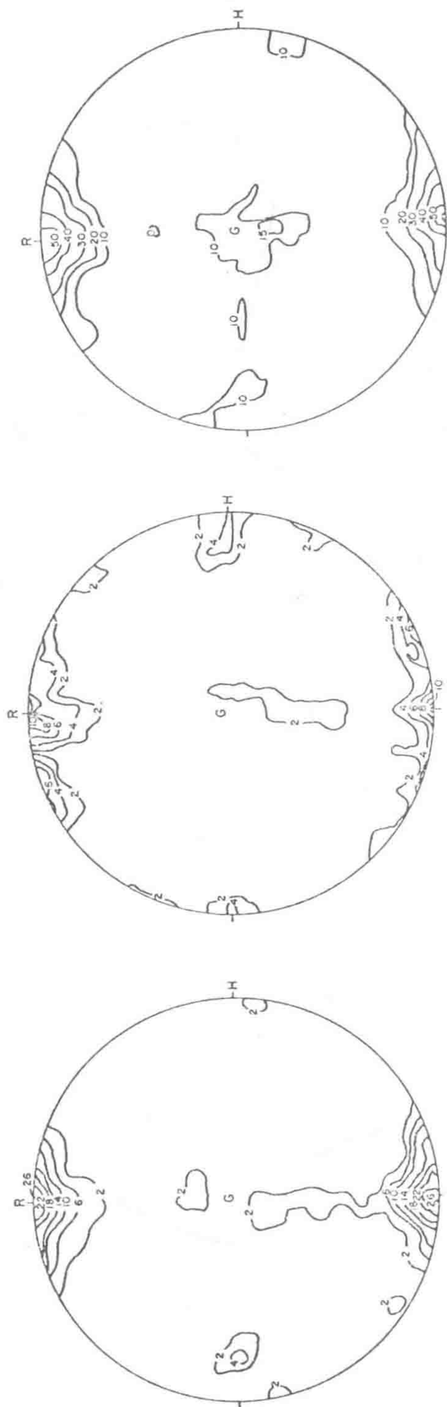
FIG. 3. Stereonet contour diagrams of frequency of poles to microcracks in Chelmsford granite. Equal-area net was used as base. (a) Transgranular microcracks in quartz. (b) Transgranular microcracks in feldspar. (c) Composite of all transgranular and intergranular microcracks in quartz and feldspar.
