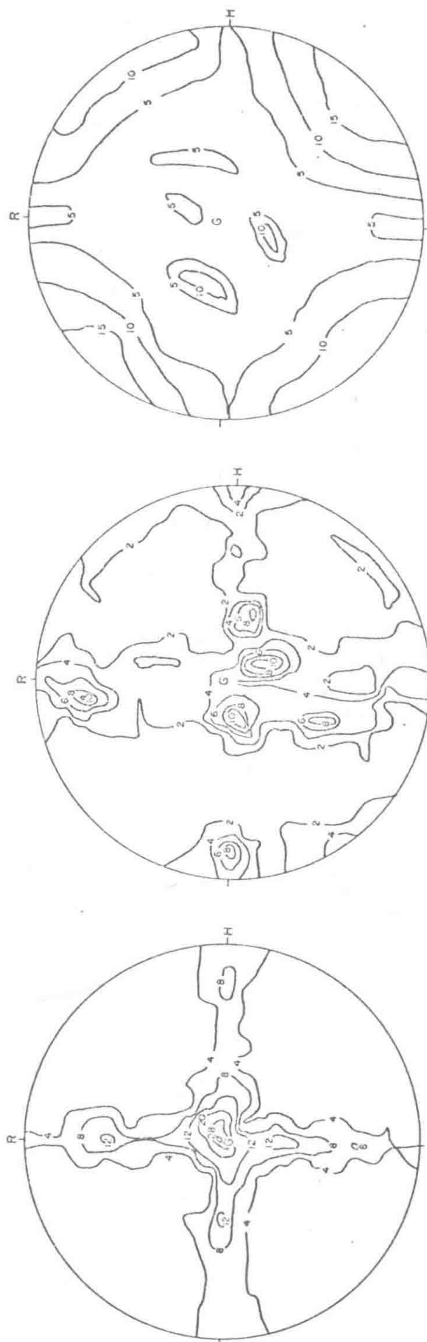
FIG. 3. Stereonet contour diagrams of frequency of poles to microcracks in Chelmsford granite. Equal-area net was used as base. (a) Transgranular microcracks in quartz. (b) Transgranular microcracks in feldspar. (c) Composite of all transgranular and intergranular microcracks in quartz and feldspar.
