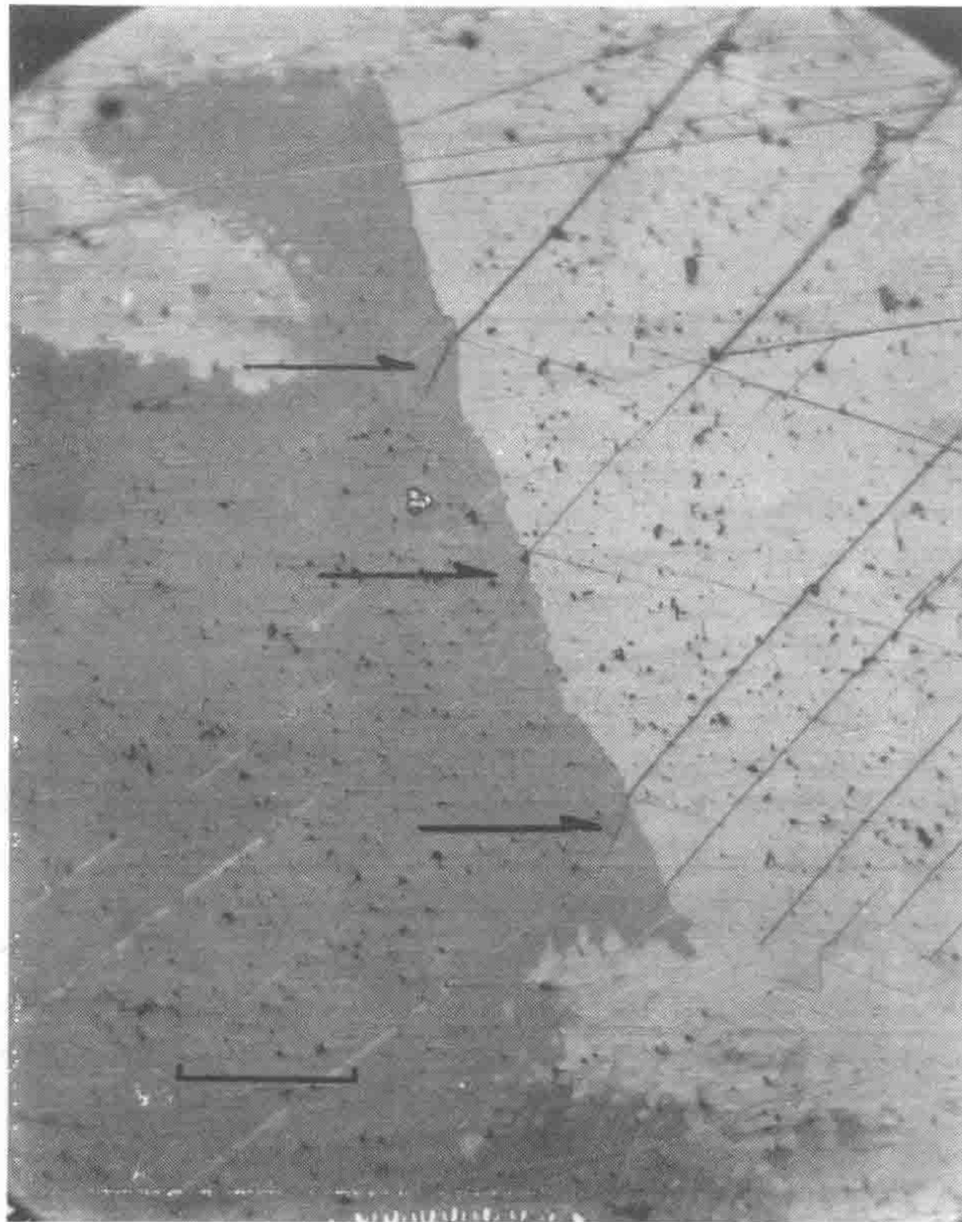
Fig. 1. Twin lamellae causing twin initiation (arrows) across a grain boundary. Maximum compression is vertical. Scale bar is 0.1 mm.
